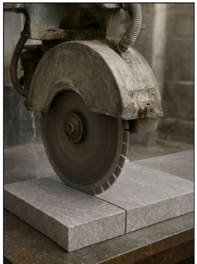
Circular diamond blade slicing slab on a bridge-saw.
